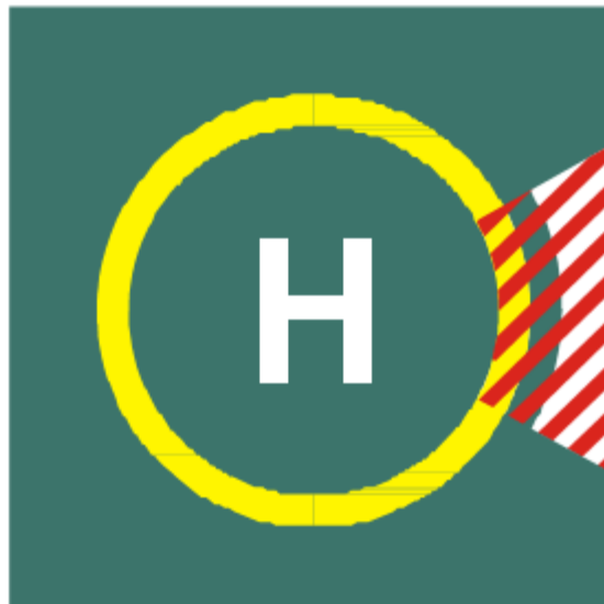
Figure 26 - Helideck prohibited landing sector marking ( ICAO Annex 14, Vol II Figure 5.1)
